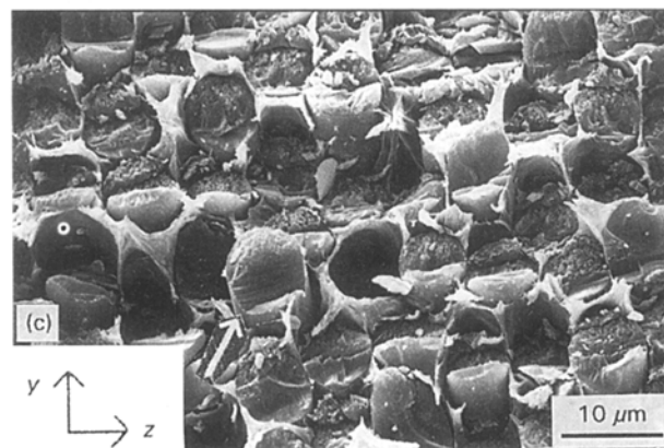
Figure 8 SEM micrographs of a fracture surface of a unidirectional composite.
